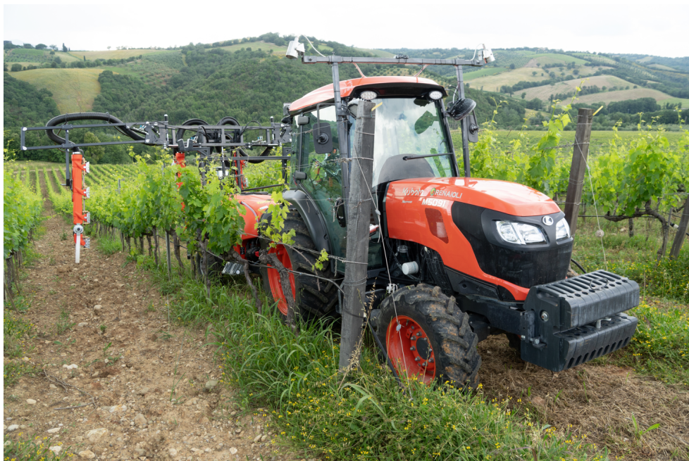
Picture: Kubota tractor equipped with Chouette sensors for scanning diseases pressure in vineyards on test farms in Italy.
